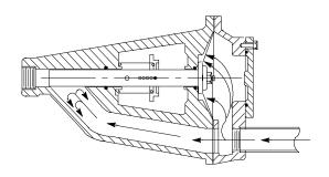
Figure 3. Valve in Closed Position
